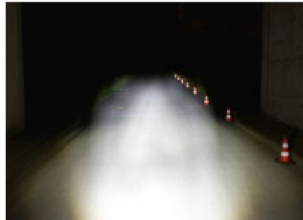
Lux values do not say all. It all depends on the light field. On the left: a nominal output of 60 Lux. On the right: "only" 50 Lux, but with light at close range and a very homogenous light field
