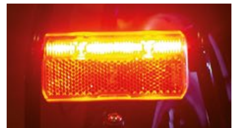
BrakeTec works only when the rear light is connected to a headlight whose rear light contacts supply alternating current.
